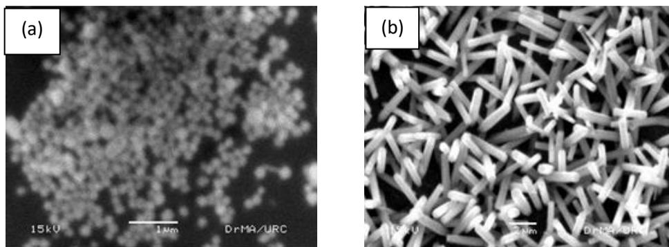
**Figure 4:**(a) Top-view SEM images of sample S1 (a) silver seed layer which is coated onetime on the glass substrate (b) ZnO nanorod which is grown on thin seed layer
