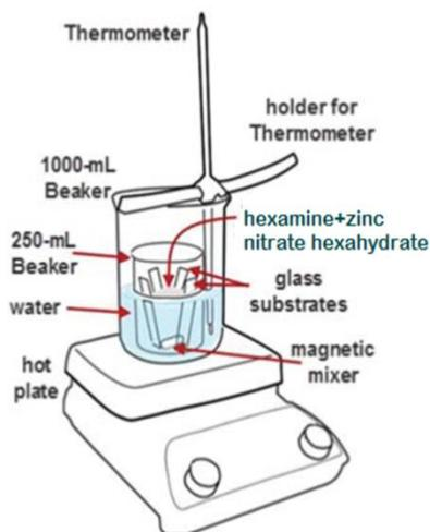
**Figure 2:** The schematic diagram of chemical bath deposition of ZnO nanostructure
