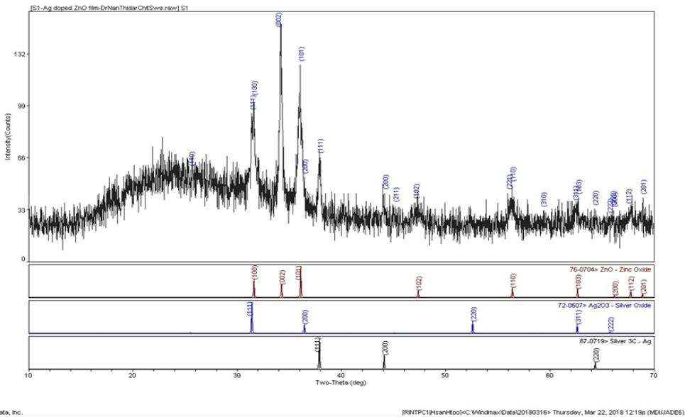
**Figure 6:** XRD plots obtained from ZnO nanostructures sample to investigate the structures and crystallinity. Reference bulk reflections of pure Ag and Ag<sub>2</sub>O<sub>3</sub> phases are shown at the bottom (ICDD-PDF#07-0719), (ICDD-PDF#72-0607).
