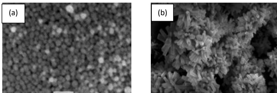
**Figure 6:** (a) Top-view SEM images of sample S3 (a) silver thick seed layer which is coated three times on the glass substrate(b) ZnO nanoflowers which is grown on thicker seed layer.
