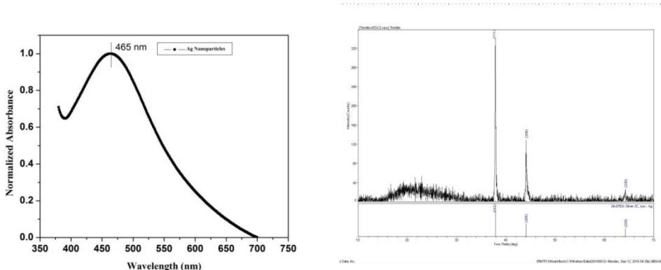
**Figure 3 :**(a) UV-Vis spectra of silver nanoparticle in which the absorptions at 465 nm were attributed to the plasmon resonance peaks of silver
