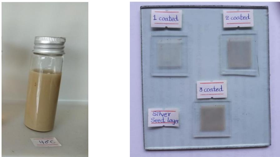
**Figure 1:** (a) Silver nanoparticle (b) Silver nanoparticles seed layer coated on glass slide
