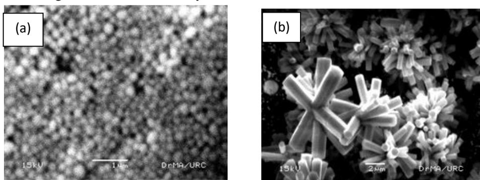
**Figure 5:** (a) Top-view SEM images of sample S1 (a) silver thickseed layer which is coated two times (b) ZnO nanorod which is grown on thicker seed layer
